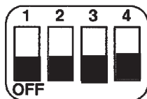
Figure 3-2: DIP Switch Block with Read After Write Disabled (Switch #2 OFF)
